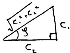
$$\sin \varphi = \frac{C_1}{\sqrt{C_1^2 + C_2^2}}$$
