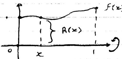
$$\begin{aligned} R(x) &= \sqrt{x^2 + 1} \\ \text{Volume} &= \pi \int_0^1 R(x)^2 dx = \pi \int_0^1 (x^2 + 1) dx \\ &= \pi \left( \frac{x^3}{3} + x \right) \Big|_0^1 = \frac{4\pi}{3} \end{aligned}$$
