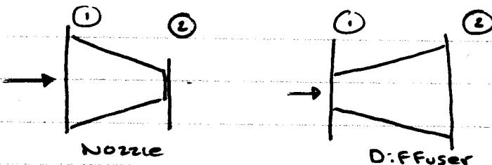
$$\dot{m}(h_2 + \frac{V_2^2}{2} + gz_2) = \dot{m}(h_1 + \frac{V_1^2}{2} + gz_1)$$
