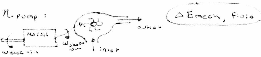
$$\eta_{\text{pump}} = \frac{\Delta E_{\text{mech, fluid}}}{W_{\text{shaft, in}}}$$
