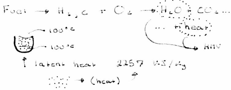
$$\eta_{\text{combustion}} = \frac{Q}{HV} = \frac{\text{Amount of heat released during comb.}}{\text{Heating Value of Fuel Burned}}$$
