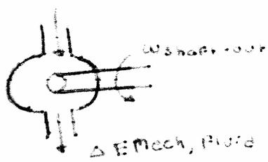
$$\eta_{\text{turbine}} = \frac{W_{\text{shaft, out}}}{\Delta E_{\text{mech, fluid}}}$$
