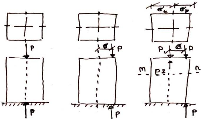
$$\sigma_c = \frac{PeC_c}{I} + \frac{P/A}{\text{---}} \quad / \quad \sigma_t = \frac{PeC_t}{I} - \frac{P/A}{\text{---}}$$
