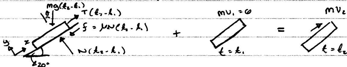
In the y-direction:  $0 + N(t_2 - t_1) - mg(\cos 20^\circ)(t_2 - t_1) = 0$
