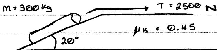
Determine the time for the log to reach a speed of 0.5 m/s. Starting from rest.
