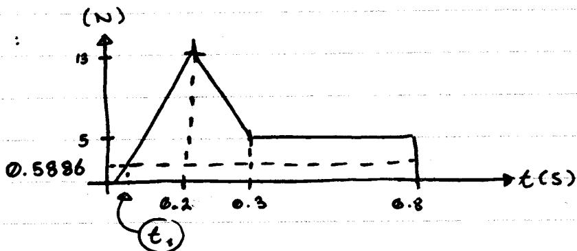
$$M V_1 + I_{\text{Imp},1 \rightarrow 2} = M V_2$$
