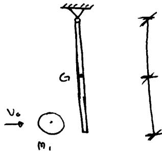
Draw the impulse-momentum diagram for the ball and the bar separately. Time 1 is immediately before the impact and time 2 is immediately after.
