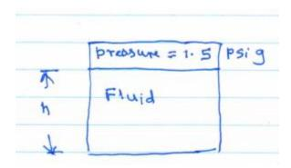
A convenient method to deal with such situations is to use the concept of piezometric head, in which the actual pressure above the fluid,  $P_A$ , is converted into an equivalent depth of the fluid,  $h_a$ , that would create the same pressure.
