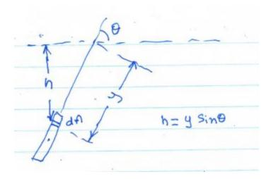
Because the area is inclined at an angle  $\theta$ , it is convenient using y to denote the position of area at any depth, h.
