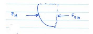
The area on which  $F_{2b}$  acts is the projection of the curved surface on the vertical plane.
