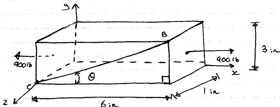
The angle  $\theta$  decreases by  $\Delta\theta 0.01^\circ$  after the load is applied. Find the Poisson's ratio,
