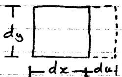
$$\epsilon_x = \frac{du}{dx} = \text{normal strain of a line segment in } x\text{-direction}$$
