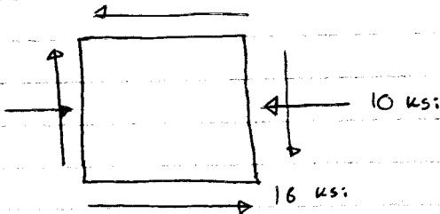
Find the equivalent state of stress on an element if it is oriented  $30^\circ$  CCW from the element shown.
