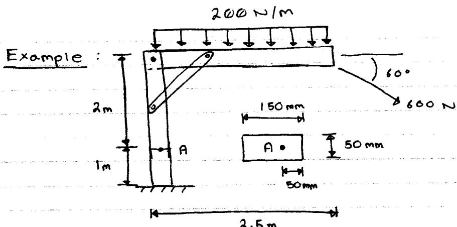
Determine the principal stresses and the max in-plane shear stress at A.
