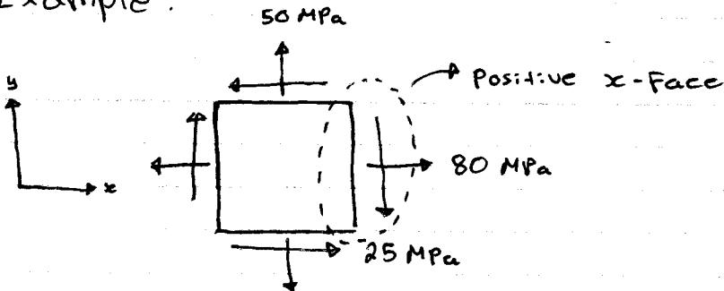
Determine the state of Stress at the point on another element oriented  $30^\circ$  cw from the position shown.
