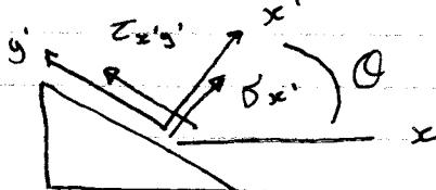
$$\begin{aligned}\sigma_{x'} &= \sigma_x \cos^2\theta + \sigma_y \sin^2\theta + 2\tau_{xy} \sin\theta \cos\theta \\ \tau_{x'y'} &= -(\sigma_x - \sigma_y) \sin\theta \cos\theta + \tau_{xy} (\cos^2\theta - \sin^2\theta) \\ \theta &= 0^\circ, \quad \cos\theta = 1, \quad \sin\theta = 0\end{aligned}$$
