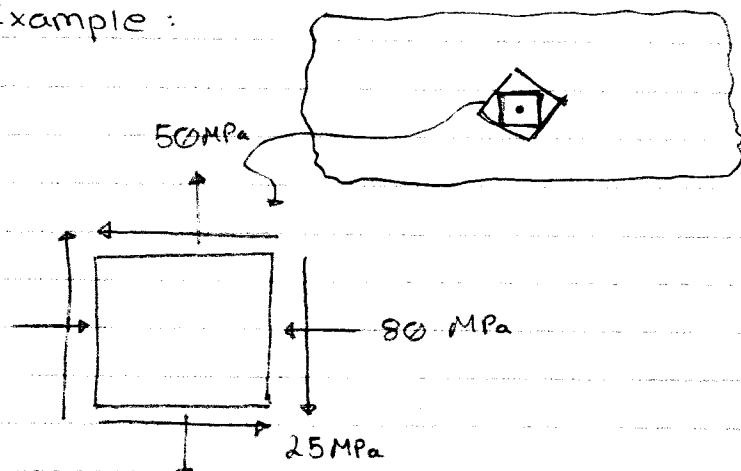
Find the state of stress at the point on an element oriented  $30^\circ$  c.w. from this position.
