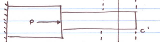
$$\delta_P = \frac{F_{AB} l_{AB}}{E A_{AB}} \\ \Rightarrow \frac{(200 \cdot 10^3 \text{ N})(0.6 \text{ m})}{(200 \cdot 10^9 \text{ Pa})(\pi/4(0.005)^2)}$$
