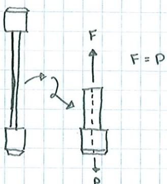
Force  $P$  (measured by load cell)
