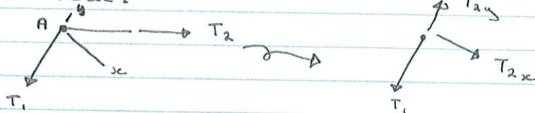
Because the sum of the forces in the x-direction must equal zero,  $T_{2x} = 0 \therefore T_2 = 0$
