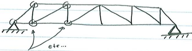
Method of Joints - Analyzing each individual joint sequentially.
