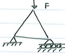
We can construct more elaborate structures by adding more triangles. The bars are the members of these structures, and the places where the bars are pinned together are called the joints. If these structures are supported and loaded at their joints, and we neglect the weight of the bars, each bar is a two-force member. Such a structure is called a truss.
