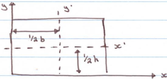
Determine the moment of inertia in terms of the  $xy$  coordinate system.
