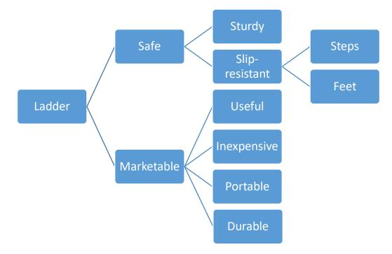
Example objective tree for ladder design (added constraint in green):
