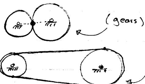
how motion is transmitted from one rigid body to another, based on the "no slip" assumption
