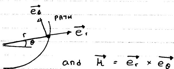
$$\left. \begin{aligned} \sum F_r &= m a_r \\ &= m(r\ddot{i} - r\dot{\theta}^2) \\ \sum F_\theta &= m a_\theta \\ &= m(r\ddot{\theta} + 2\dot{r}\dot{\theta}) \\ \sum F_z &= 0 \end{aligned} \right\}$$
