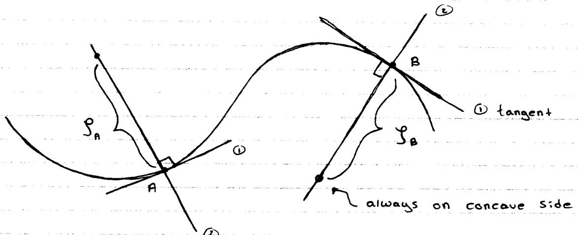
Planar motion (tangential - normal components)
