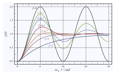
Critical damping exists between the overdamped and underdamped cases, where the system returns to equilibrium in the minimum amount of time – the system fails to overshoot and not a single oscillation is made.
