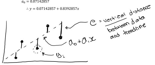
Estimate of the linear regression (error from the sampling data to the straight line):
