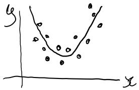
data:  $y = a_0 + a_1 x + a_2 x^2 + e$   $y = a_0 + a_1 x + a_2 x^2 + e$   $when constant <math display="block">e_i^2 = \sum (y_i - a_0 - a_1 x_i - a_2 x_i^2)^2$ Where the data cannot be represented by a linear line of best fit, so a second order polynomial (quadratic) line of best fit can be used.
