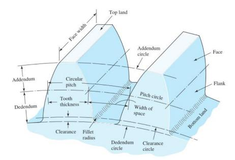
**Tooth System:** refers to the standard that specifies the tooth geometry and so on. There are the metric system and the US customary system.
