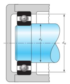
$d_{\rm S}$  is the shaft shoulder diameter. Catalogs may list the min and max values of  $d_{\rm S}$ . If only one value is given, it is typically the minimum value.
