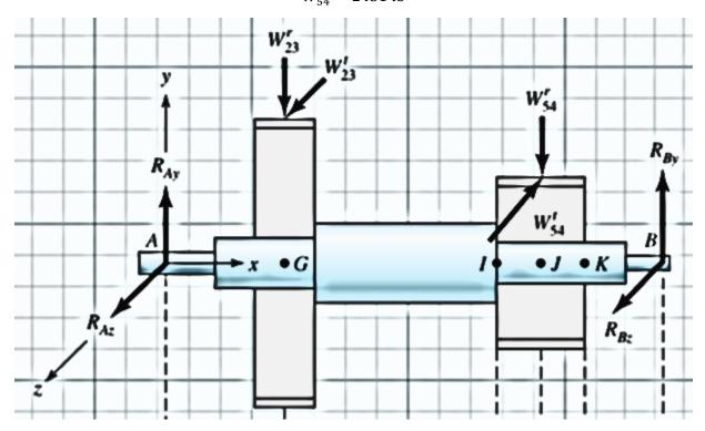
We are to select appropriate materials and/or diameters at various cross sections, based on fatigue with infinite life. Design factor is 1.5.
