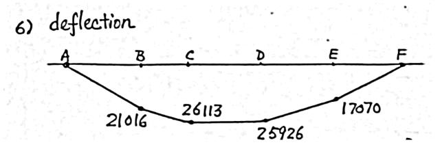
To obtain deflection curve of step (6), at any cross-section, subtract value obtained in step (4) from baseline value.
