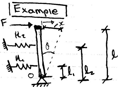
Find the equivalent stiffness of the system that relates the applied force to the resulting displacement  $x$
