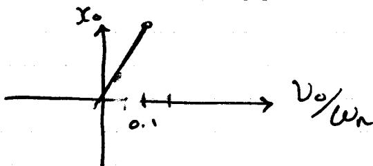
b)  $\phi = \tan^{-1}\left(\frac{\omega_n x_0}{v_0}\right) = \tan^{-1}\left(\frac{(10)(-2)}{1}\right) = -1.521 \text{ rad}$
