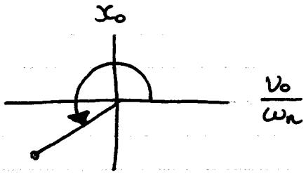
$$x(t) = \frac{\sqrt{\omega_n^2 x_0^2 + v_0^2}}{\omega_n} \sin\left(\omega_n t + \tan^{-1} \frac{v_0 x_0}{\omega_n}\right)$$
