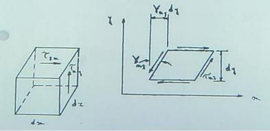
$$dU_{shear} = \left(\frac{1}{2}\right)\tau_{xy}\;dx\;dz\cdot\gamma_{xy}\;dy = \left(\frac{1}{2}\right)\tau_{xy}\;dv\;\gamma_{avg}$$
