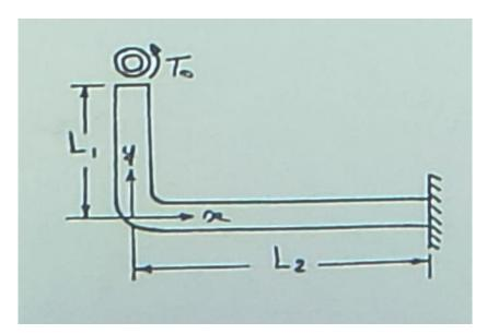
Length  $L_1$  of pipe is subjected to torque  $T_o$
