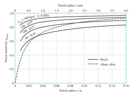
The notch sensitivity of cast iron is very low. However, to be on the conservative side, it is recommended that q=0.20 be used for all grades of cast iron.
