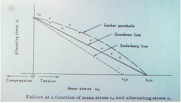
In this particular graph, if the  $SAE\ No$ . or the ultimate strength is known, and if N is known (number of cycles). The fatigue or endurance limit of the material can be found. However, the above data is for zero mean stress  $S_m=0$ . To solve for cases where  $S_m\neq 0$ , first  $S_A-N\ Cures$  are plotted as shown. Then for a given  $N=N_1$  the  $S_a=S_m$  curve is plotted.
