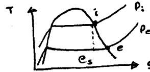
Efficiency of compressor / pump
