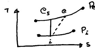
Efficiency of a cooled compressor
