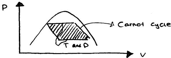
In a cylinder/piston system involving boundary-movement work:  $W_{\text{net}} = \int_1^2 P dv + \int_2^3 P dr + \int_3^4 P dv + \int_4^1 P dv$
