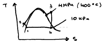
$$\text{Pump: } w_p = -V(P_3 - P_1) \\ = -0.001001(4000 - 10) \\ w_p = -416.5 \text{ kJ/kg}$$
