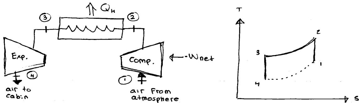
Air refrigeration cycle utilizing a heat exchanger
