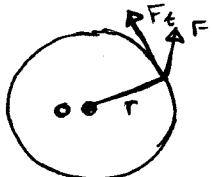
$$\text{Magnitude of torque: } M = I_{mass} r^2 \alpha \delta m$$
