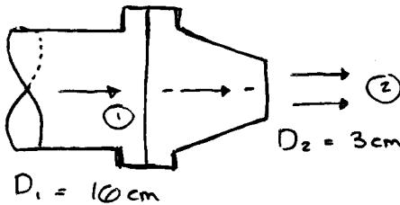
$$Q = 1.5 \text{ m}^3/\text{min} = 0.025 \text{ m}^3/\text{s}$$
