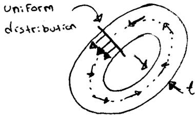
$$q = \tau t \text{ (shear flow)}$$
