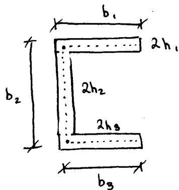
$$\begin{aligned} J &= l_3 (2h_1)^3 (b_1) \\ &+ (l_3)(2h_2)^3 (b_2) \\ &+ (l_3)(2h_3)^3 (b_3) \end{aligned}$$
