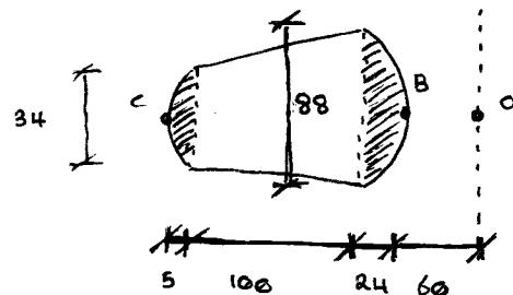
Find the max load the crane hook can support
