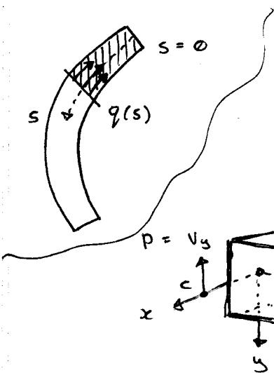
Example: Determine the shear flow in a C channel section due to a shear force  $V_y$  through its shear center.
