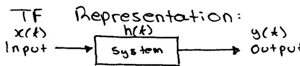
$$\left. \begin{aligned} y(t) &= h(t) \otimes x(t) \\ Y(s) &= H(s) * X(s) \end{aligned} \right\}$$
