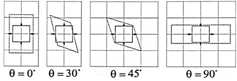
No shear strain (deformation) if angle is 0° or 90°
