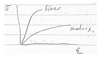
Within the section, it's assumed that  $\sigma - \varepsilon$  plots for both fiber and matrix are linear up to failure (by breakage or by fracture)
