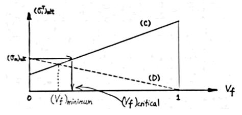
$$\left(V_f\right)_{minimum} = \frac{(\sigma_m)_{ult} - E_m \cdot \frac{\sigma_f}{E_f}}{\left(\sigma_f\right)_{ult} \left(1 - \frac{E_m}{E_f}\right) + (\sigma_m)_{ult}}$$
