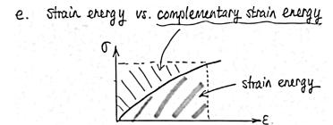
Strain energy: in terms of strains and elastic moduli
