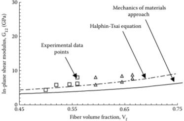
FIGURE 3.17 Theoretical values of in-plane shear modulus as a function of fiber volume fraction compared with experimental values for unidirectional glass/epoxy lamina ( $G_f$  = 30.19 GPa,  $G_m$  = 1.83 GPa). Figure (b) zooms figure (a) for fiber volume fraction between 0.45 and 0.75. (Experimental data from Hashin, Z., NASA tech. rep. contract No. NAS1-8818, November 1970.)
