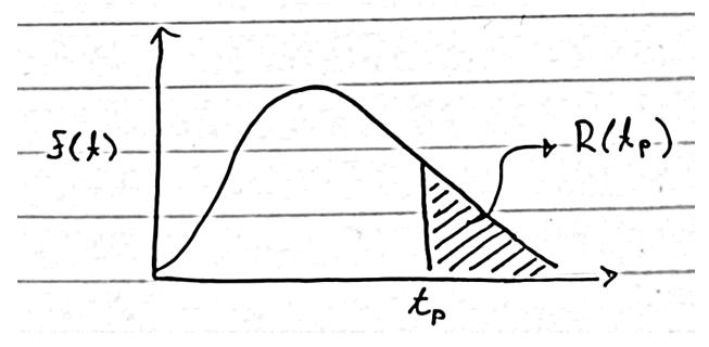
The probability of a failure cycle is the probability of failure occurring before time  $t_p$ , which is the unshaded area  $[1-R(t_p)]$
