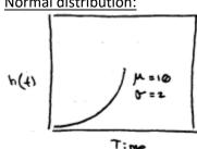
$$h(t) = \frac{\exp \left[ -(1-\mu)^{2}/2\sigma^{2} \right]}{\int_{t}^{\infty} \exp \left[ -\frac{(1-\mu)^{2}}{2\sigma^{2}} \right] dt}$$
