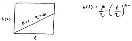
When the hazard rate increases with time, such as for the normal and Weibull distribution, it indicates an aging or wear-out effect.
