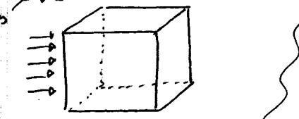
$$\begin{cases} c = c_0 & 0 < x < \infty \\ \text{at } t = 0 & @ x = 0 \\ \text{at } t > 0 & @ x = \infty \end{cases} \quad \begin{cases} c = c_s & \\ c = c_0 & \\ c = c_0 & \end{cases}$$
