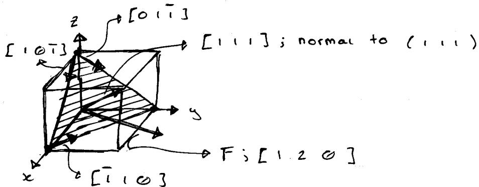
$\phi$  : angle between Force and normal to the surface
